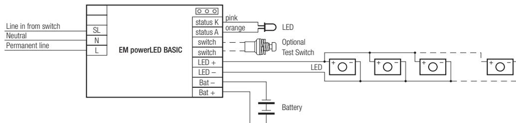
Take care that the LED is connected with the right polarity. LED that are connected to the EM powerLED devices should have a reverse polarity protection device such as a schottky diodes fitted, otherwise irreversible damage could occur if the LED is connected in reverse polarity. Any protection device must be capable of handling in excess of 700 mA.
